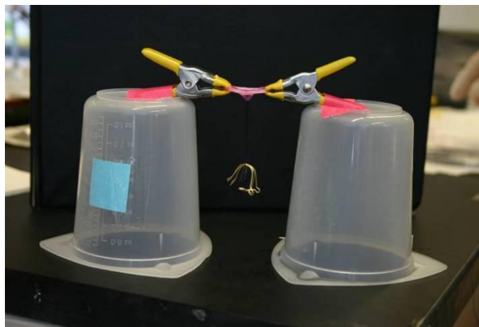
Figure 33: Collagen gel with weight added to create displacement of the gel
