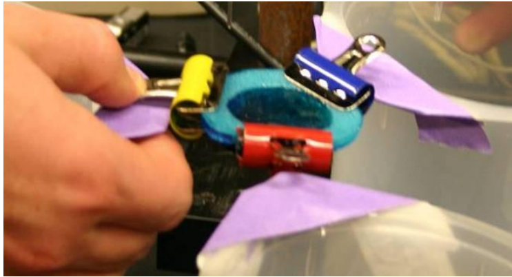
Figure 37: Mounting a sample with three binder clips
