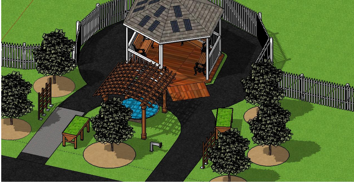
Figure 4: Finalized landscape architectural design for Gazebo area. This design features two vertical gardens, two elevated garden beds, a circular fountain, and a pergola.
