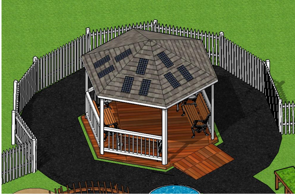
Figure 5.2.6: Example of small solar panels attached to gazebo roof
