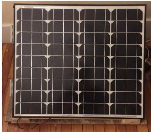
Figure 3.14: The monocrystalline solar panel mounted on the stand alone system.
