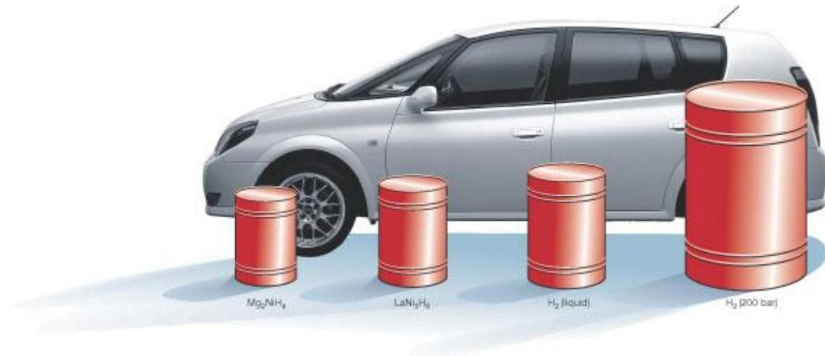
Figure 2.7. Tank volumes for various storage options for 4 kg of hydrogen on board a car (Schlapbach and Züttel, 2001).
