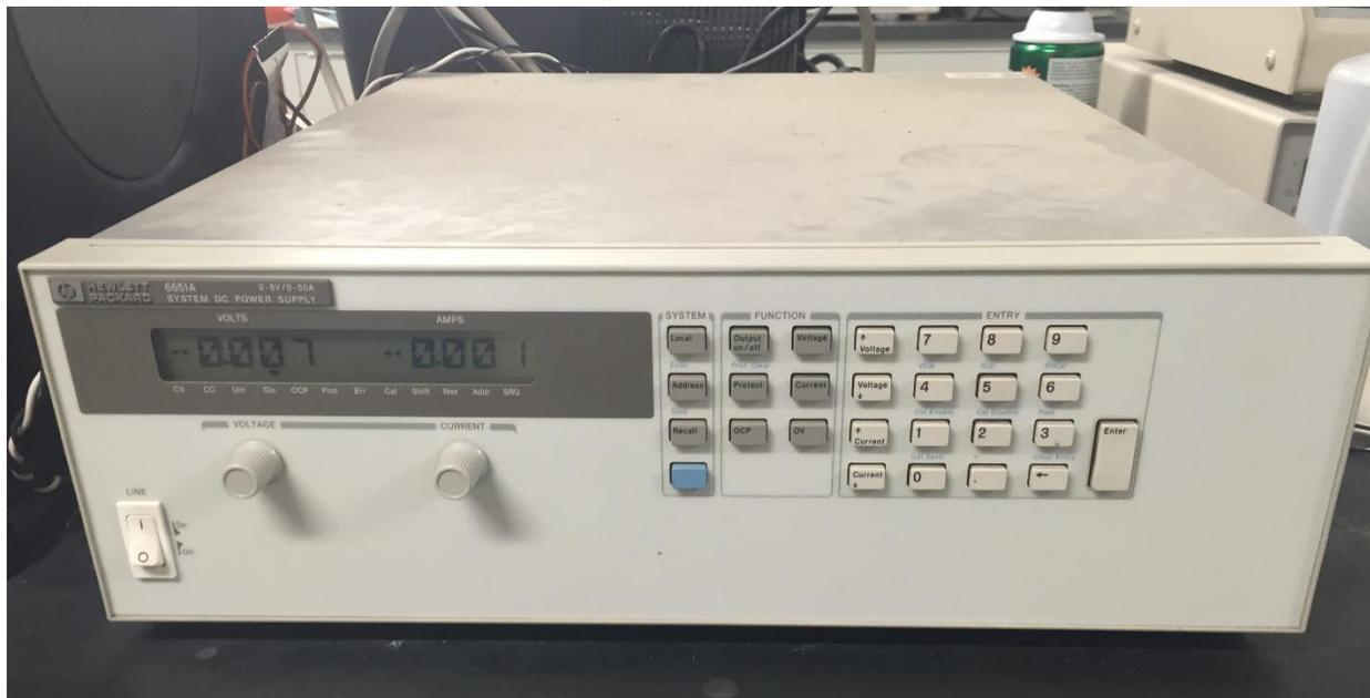
Figure 3.11: Power supply used during FCC testing.
