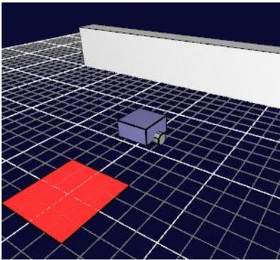
Now it's time to sense our environment. This virtual robot has a range-finding sensor on the front which will allow you to program the robot to avoid crashing into walls. To use the range-finding sensor, use the "`getFrontRange()`" function. This will return the distance to the closest wall directly in front of your robot. Here is an example:
