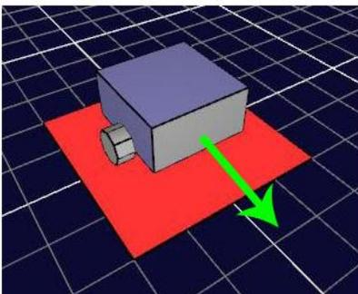
The picture to the left is your virtual robot. The front of the robot is colored grey as seen in the picture. It has 2 drivable wheels, which we will use to move the robot around the simulation. In order to do this, we will need to program the wheels to turn. You will use the `setLeftMotor(percentage)` and `setRightMotor(percentage)` functions to control the wheels. `percentage` should be a value from -100 to 100. Here are some examples:
