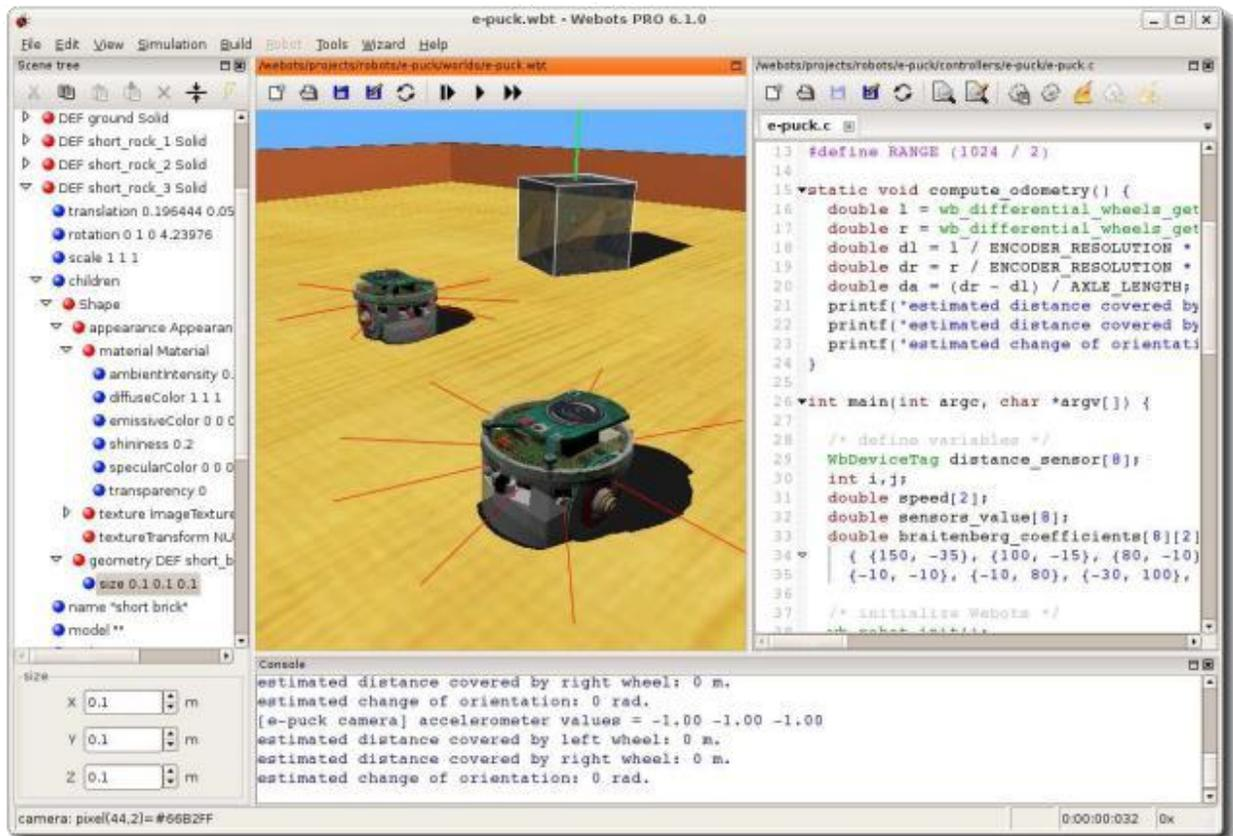
Figure 3: A virtual robot inside of Webots<sup>13</sup>
