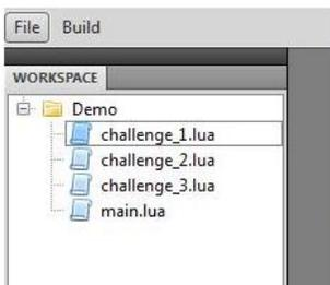
**Step 1:** Open the file called `challenge_1.lua`. The file contains 2 functions, `behavior_1()` and `DriveForward()`. `behavior_1()` is completed for you, but `DriveForward()` is empty.
