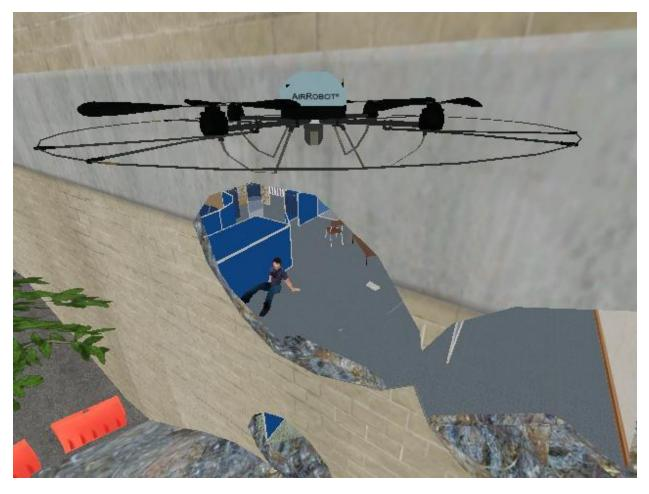
Figure 4: Aerial Robot looking inside a building using USARSim<sup>14</sup>
