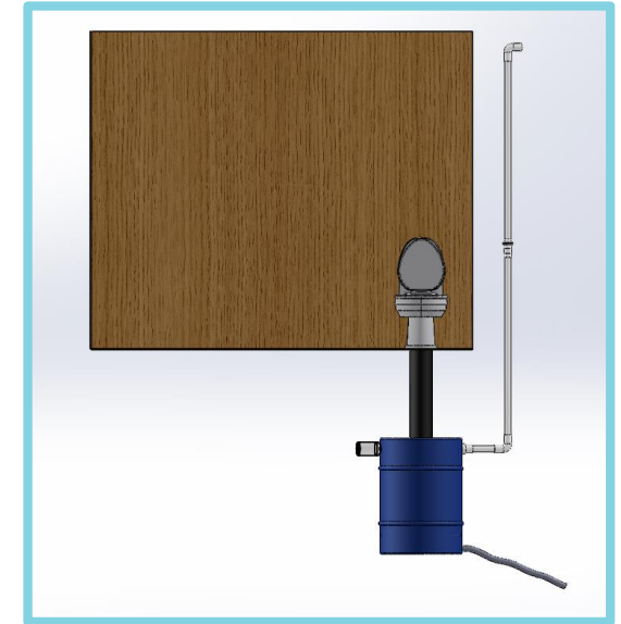
[A representation of a composting toilet system]
