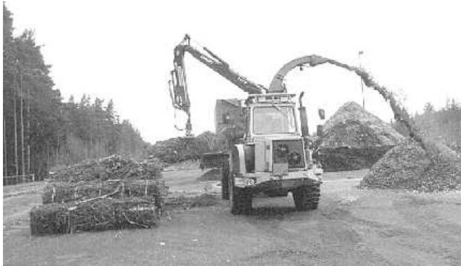
Figure 35: A Bruks 1004 CT drum chipper used to chip CRLs
