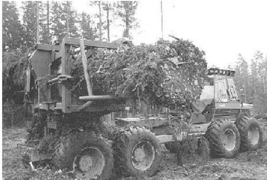
Figure 34: The Fiberpac 370, used to efficiently create CRLs
