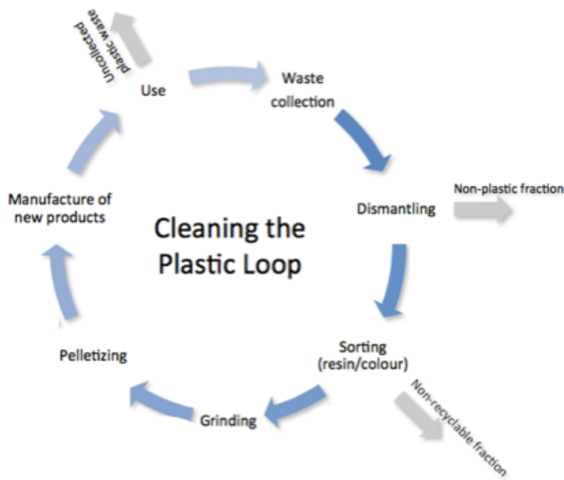
Figure 15: Plastic recycling process (adapted from Haarman, 2015)
