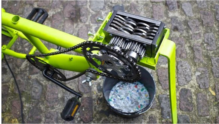
Figure 27: "The Ingenio" bicycle-powered plastic shredder (Holaciudad, 2013)
