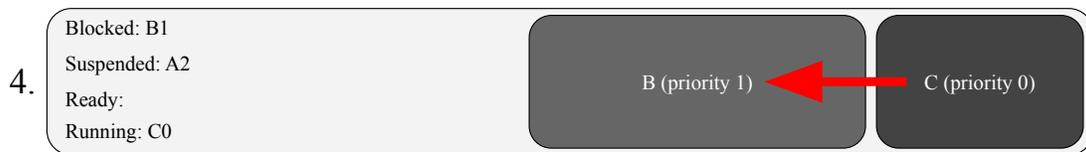
Figure 3.4: A violation of [requirement 1](#) or [requirement 2](#) would cause a lower priority task to corrupt the stack of a higher priority one.
