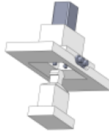
Figure 15: Custom Electrical Connection using touch latches. 30
