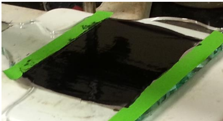
Figure 3-6: Aluminum foil coated with active cathode material.
