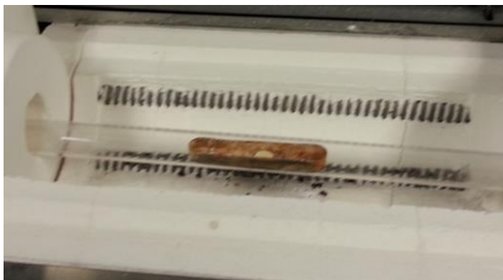
Figure 3-3: Calcination of cathode precursor material.
