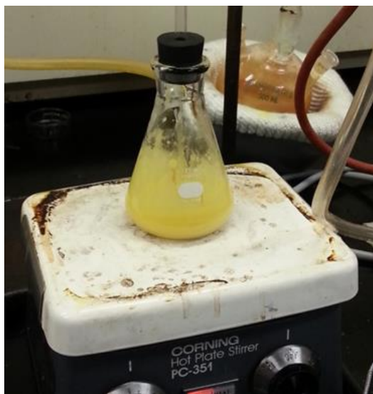
Figure 3-2: Mixing of solution to form gel under nitrogen flux using stirring rod.
