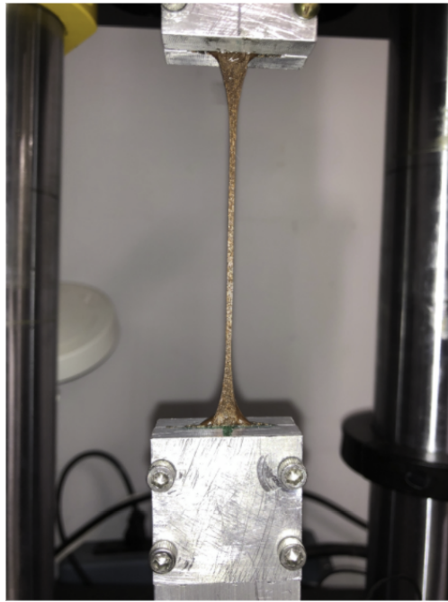
Figure 4.18.: One of the mixed dogbone samples under tensile testing on the Instron.
