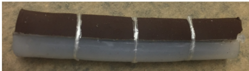
Figure 4.15.: The Three-Ringed Constraint Design.
