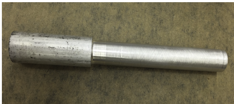
Figure 4.11.: Aluminum Mandrel for Actuator Half-Bonding.
