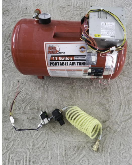
Figure 4.21.: The air tank, power source, and pressure regulators.
