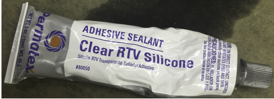
Figure 4.13.: Silicone Adhesive for Bonding the Actuator Halves.
