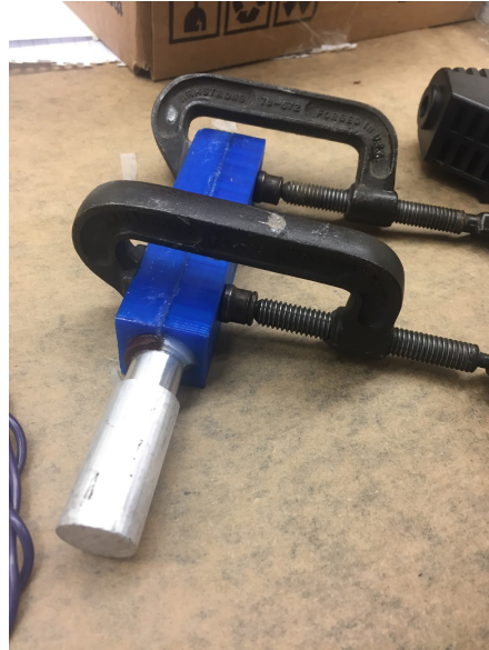
Figure 4.14.: The Setup for Bonding the Two Halves of the Actuator.
