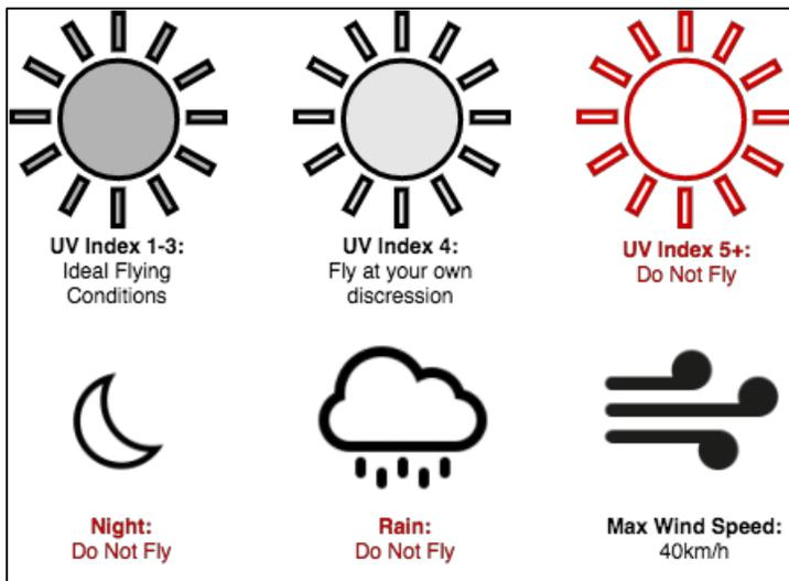
*Figure 7. Reference guide for when drones can be flown in adverse conditions. Graphics by Oliver Simon.*
