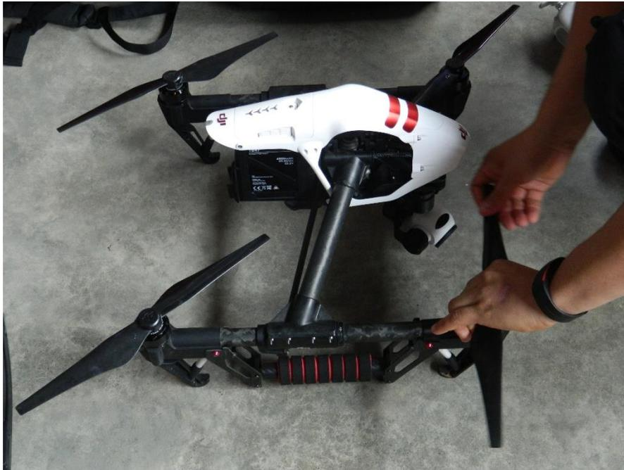
*Image 3. Steps 7 and 8: Fastening blades to the drone*
