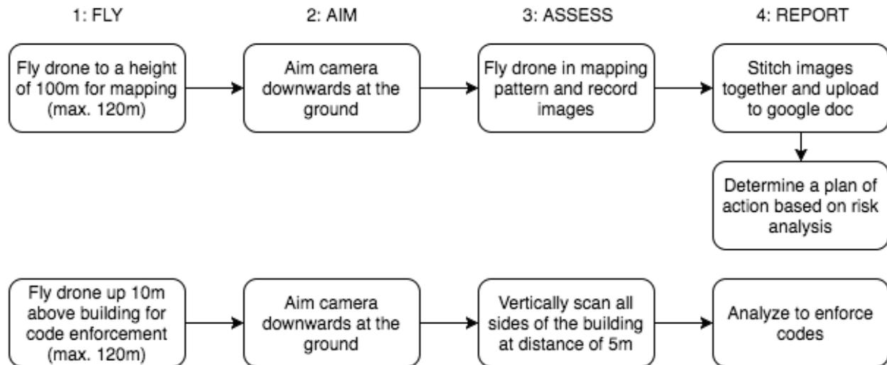
Figure 11. Flowchart to follow during a remote sensing
