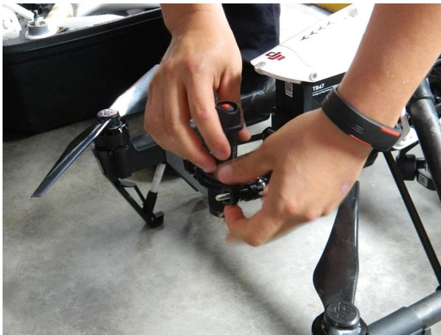
*Image 4. Step 9: Place light on rear of drone and fasten in place*
