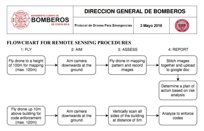
Figure 11. Flowchart to follow during a remote sensing
