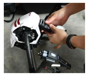
Image 2. Step 4: Place camera under front nose of drone and lock into place
