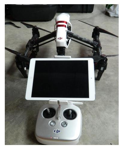
Image 5. Step 13: Place viewing device on controller stand and lock into place using clips
