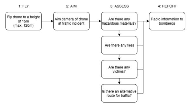
Figure 10. Flowchart to follow during a traffic incident
