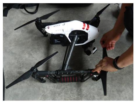
Image 3. Steps 7 and 8: Fastening blades to the drone
