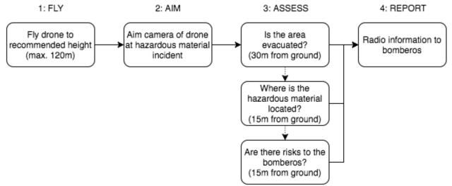
Figure 9. Flowchart to follow during a hazardous materials incident
