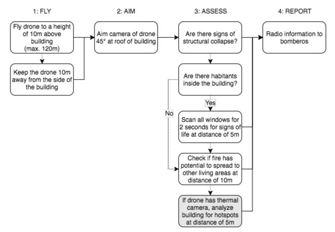
Figure 8. Flowchart to follow during a structure fire
