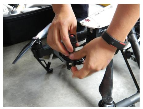
Image 4. Step 9: Place light on rear of drone and fasten in place
