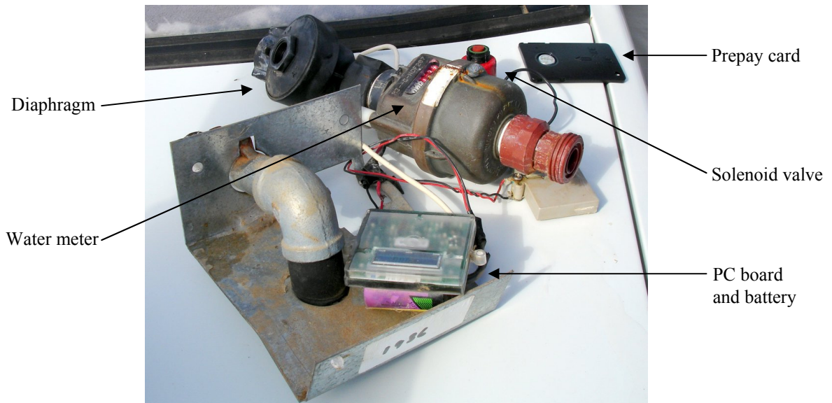
Figure 9: Inside of Prepay Meter
