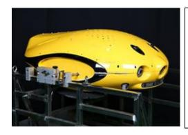
Samsung Heavy Industries' (SHI) hull cleaning robot is designed to clean SHI's LNG carriers during and immediately after production. While we were able to make contact with Samsung, they chose not to release any information on their hull cleaner.
