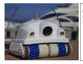
The KeelCrab Sail One was designed to clean sail boats, yachts, and maxi yachts. The robot is designed to not only clean hulls, but to also perform hull inspections.
