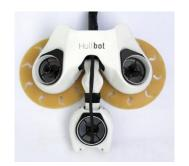
Hullbot is a hull cleaning robot primarily designed for use on yachts. It uses disk shaped rotating cleaning pads to clean vessels while at anchor. The Hullbot is designed to do a cleaning once every four hours. It uses a pre-loaded model of the yacht in order to determine its orientation as well as the percentage of surface area cleaned.
