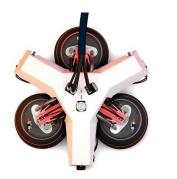
The Fleet Cleaner hull cleaning robot was developed for vessels in the shipping industry. It uses high powered water jets to remove and capture fouling.
