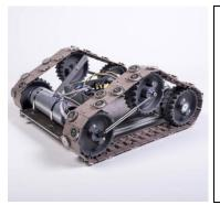
Remora is a robot in development by students at the University of Southampton. The goal of this project is to design an autonomous robot, with the ability to function and clean a ship's hull while a ship is in motion. Remora uses a hydrodynamic shell that allows the robot to function at up to 8 knots. With upgrades and further testing the students believe the system will be able to handle 15 knots.
