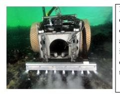
Magnetic Hull Crawler or MHC was designed with the commercial shipping industry in mind, as well as the offshore oil and gas industries. The system has been in use since 2005, and was originally designed for the purpose of hull inspection. In addition to hull cleaning, MHC can provide detailed models of hulls, pipelines and rigs. This allows users to detect issues The cleaning system is able to reach up to 1000 bar.
