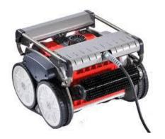
Hulltimo is designed primarily for sailboats and motorboats. It comes equipped with a camera and remote control with a display. The robot must be controlled by a trained operator, and is able to clean a 34-foot boat in approximately an hour. The suction system installed on the robot allows it to move along sharp angles on the hull surface.
