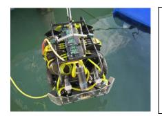
The Hull Bio-Inspired Underwater Grooming System (HullBUG) is a hull cleaner being developed by SeaRobotics and the Office of Naval Research. HullBUG is a platform that supports a diverse set of modules. It's highly adaptable and is not limited to hull cleaning. Hull integrity inspection and marine research are obvious alternate missions, though more exist.
