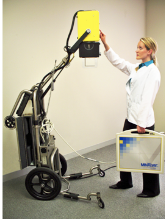
Figure 9: The CMDR-2S Portable X-ray DR System, manufactured by MinXray
