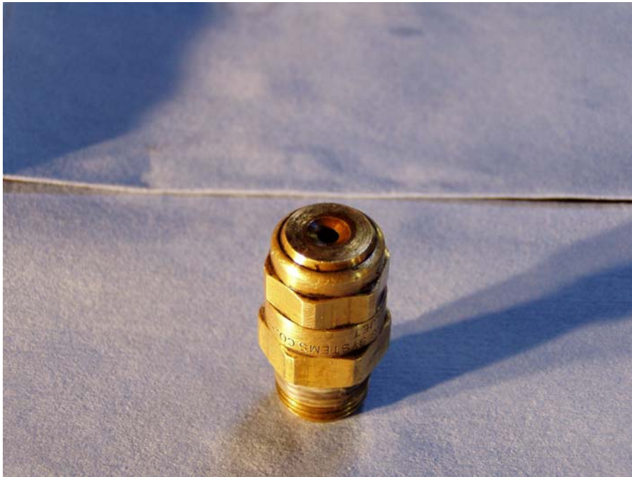
Figure 4.10 Spraying System 3/8GG, 15 nozzle.
