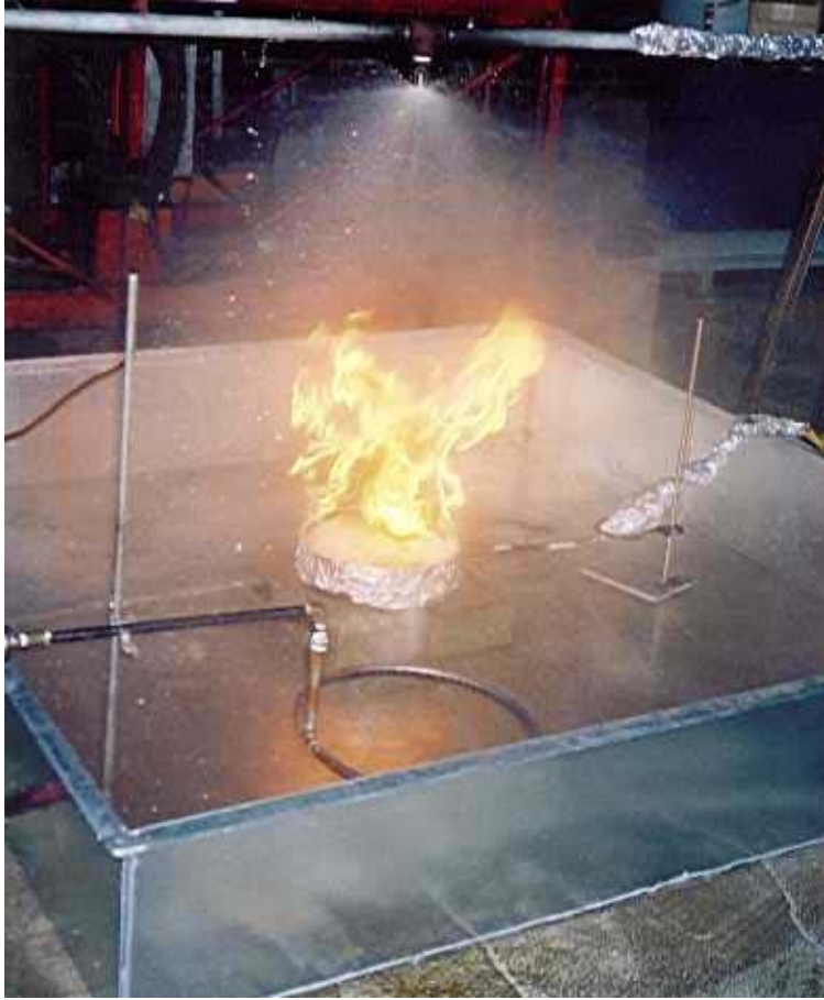
Figure 8.3 Water spray discharge onto burning oil at 7 bar for AM24 nozzle.
