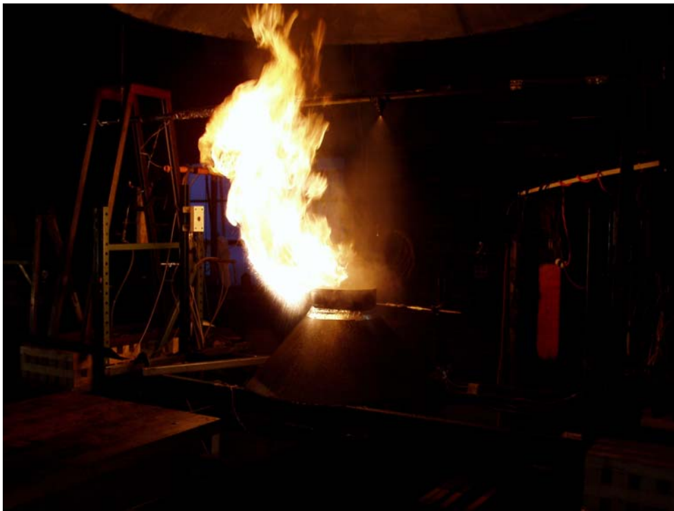
Figure 8.17 Cooking oil fire suppression test for pan 15.2 cm (6 in.) from the center of the nozzle and 91 cm (3 ft) below the nozzle.
