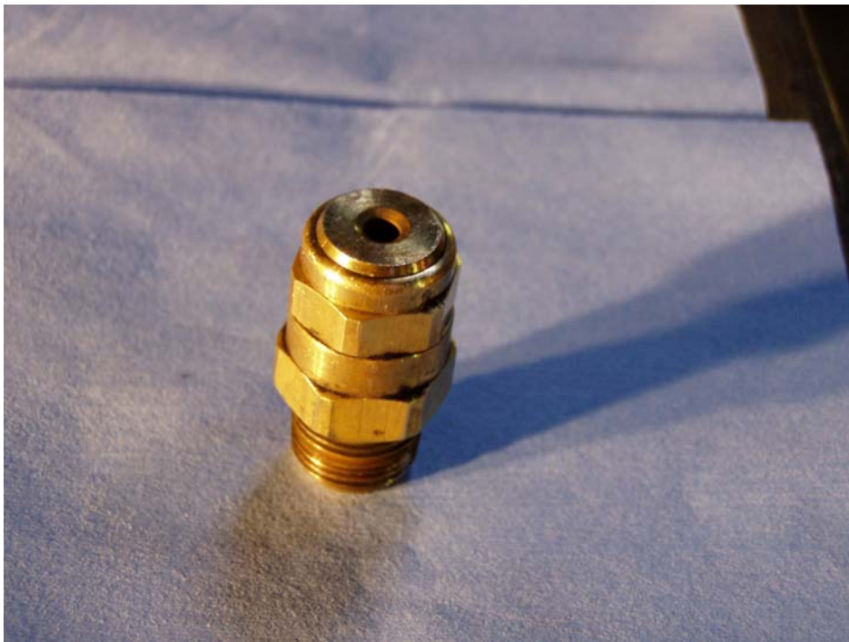
Figure 4.12 Spraying System 3/8GG, 22 nozzle.
