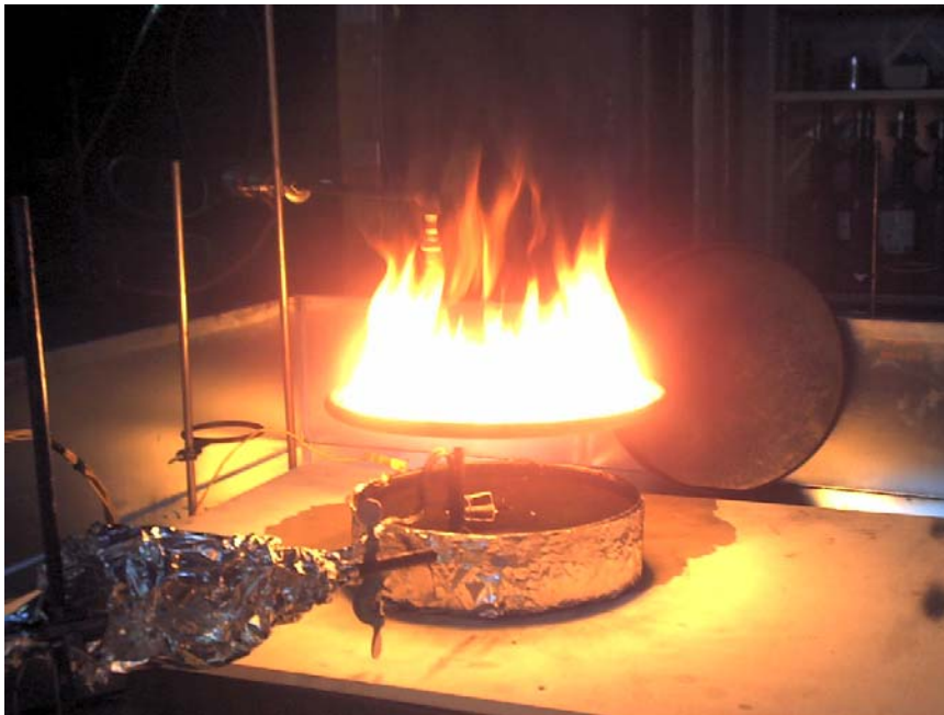
Figure 5.1 Propane ring burner used by this research to heat oil.
