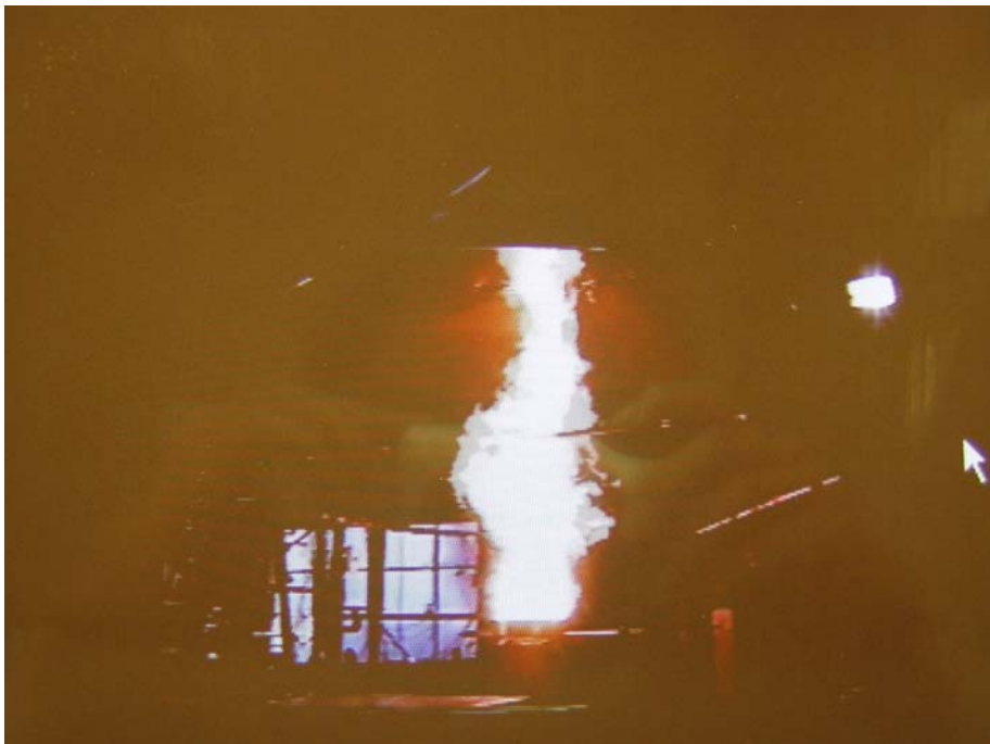
Figure 6.19 Cooking oil splattering fire for 25 psi BETE 1 1/2 water spray ( 189 \mu m ) on 270^{\circ}C oil.
