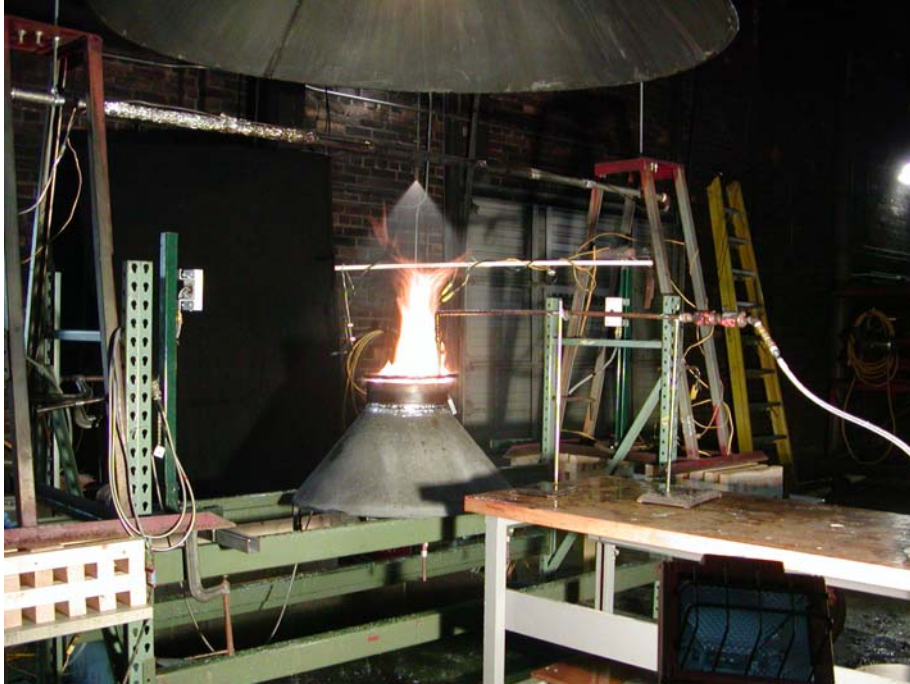
Figure B.9 Delivery Density test for 3/8GG 18SQ nozzle using 10psi water on 1.70 m^3 / hr (60 ft^3 / min ) propane fire.
