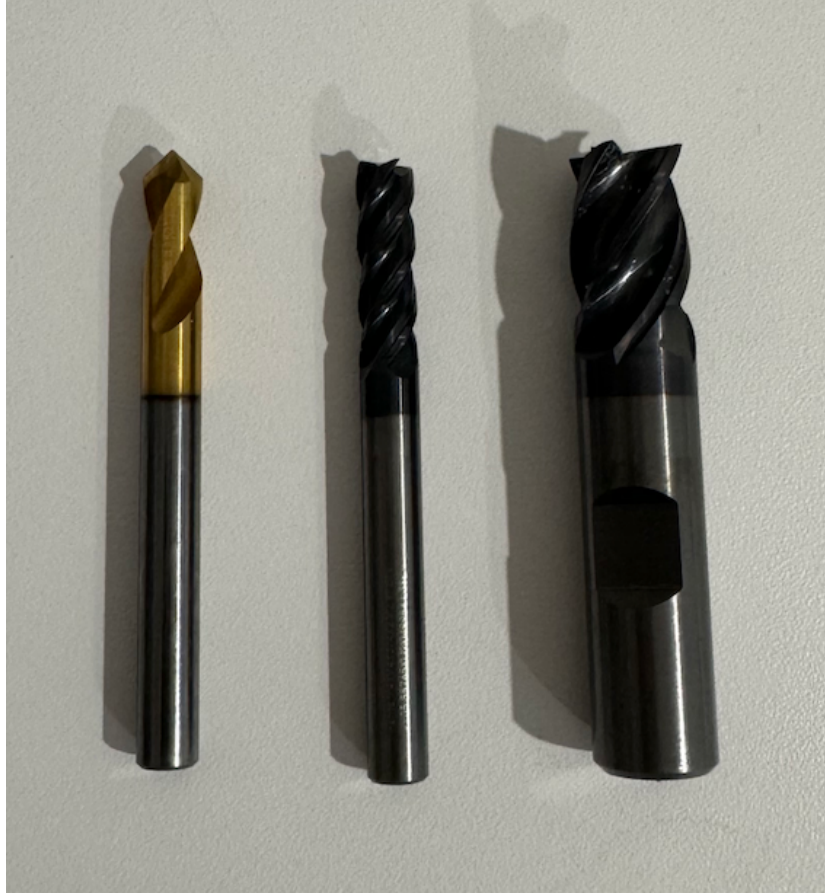
Figure 19: 1/2" Endmill 1/4" Endmill and chamfer for Steel Housing
