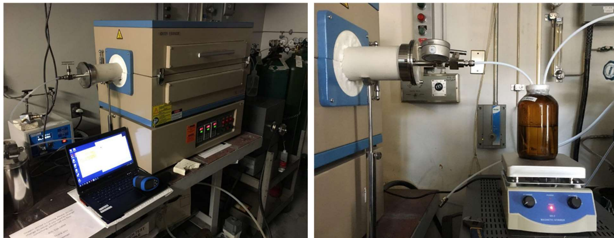
Figure 2-4. Experimental setup for heat treatment and stability tests.
