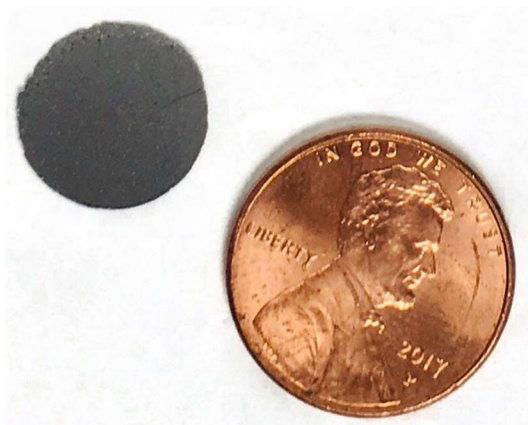
Figure 2-3. A pellet of a dual-phase composite sample after sintering at 1150°C for 2 hours under air.
