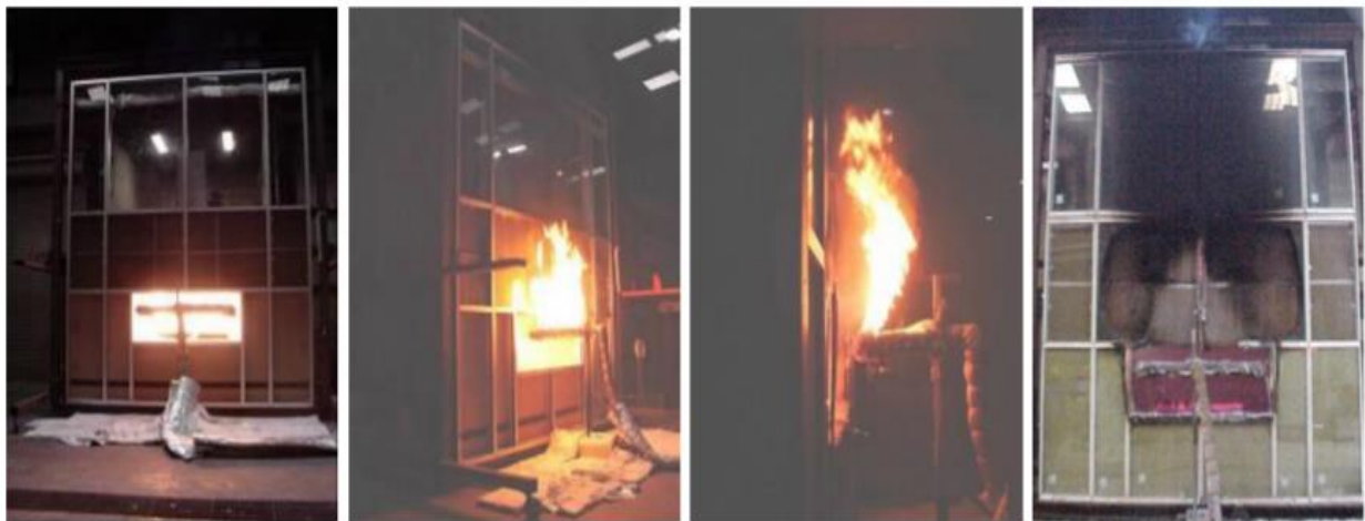
Figure 3.1: Actual Performance of ASTM E 2307 Test
