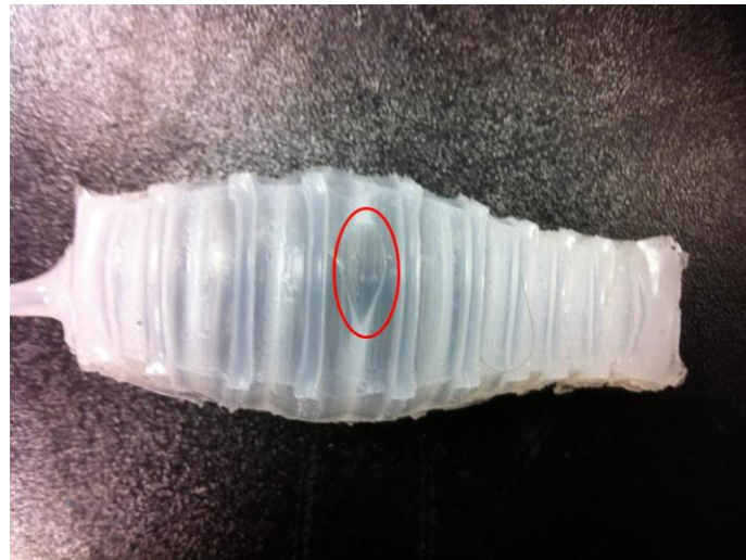
Figure 56: An Internal Structure Burst
