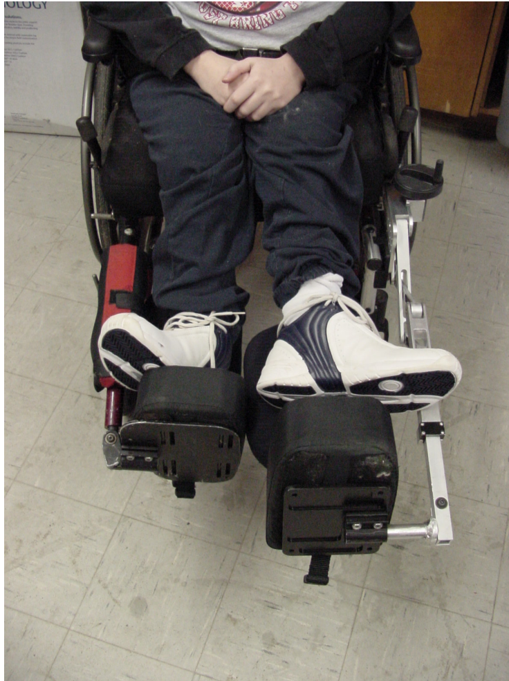
Figure 62: Test client Andy with legrests in elevated positions - the leg on the prototype legrest is able to stay straight while the leg on the original legrest is bent and rotated inward
