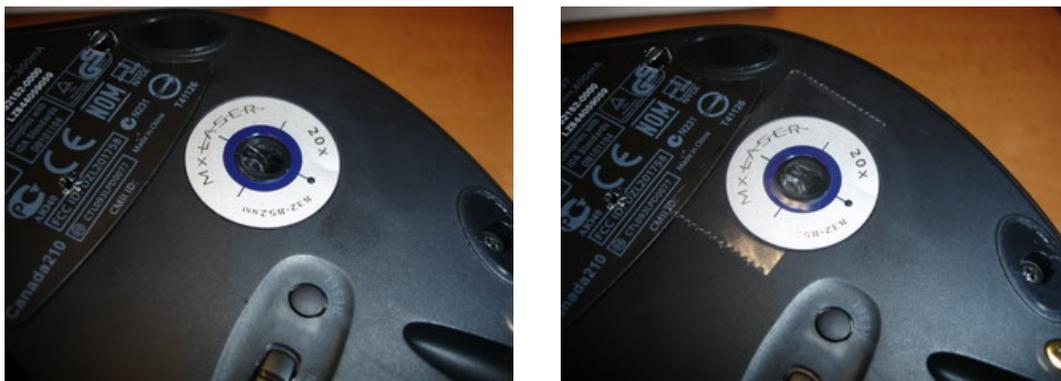
**Fig. 38 - Laser mouse without and with transparent tape mounted in front of sensor**
