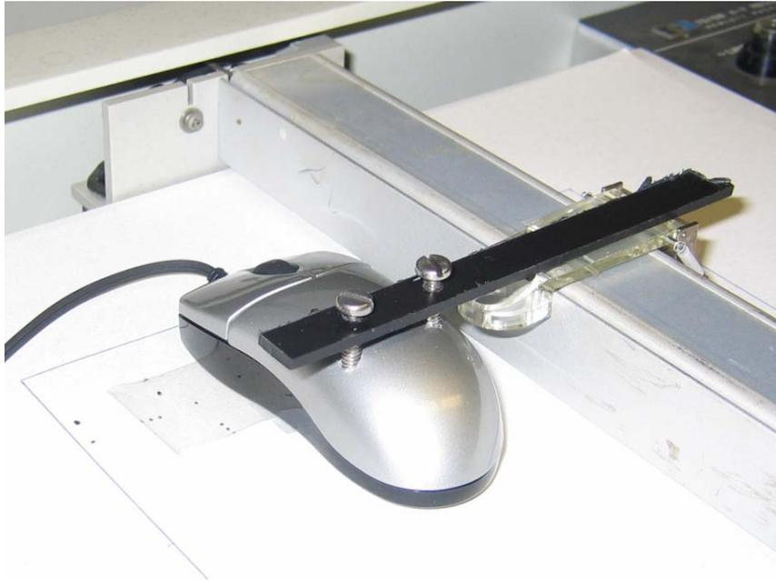
**Fig. 16 - XY recorder with mouse mounted**
