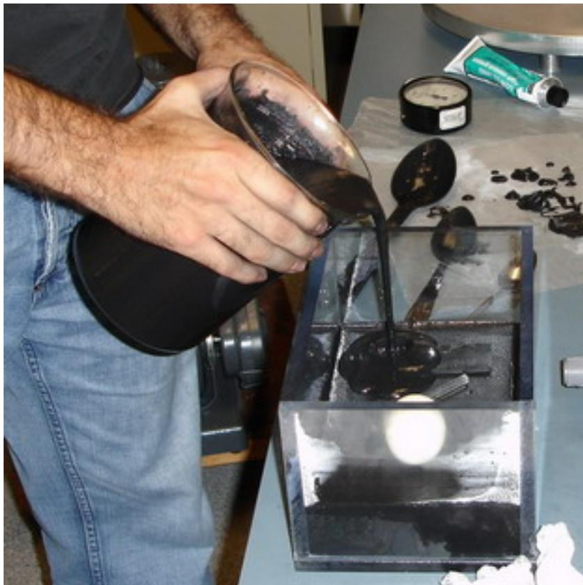
**Fig. 55 - Matt Rowan pouring agar and graphite solution into the mold**
