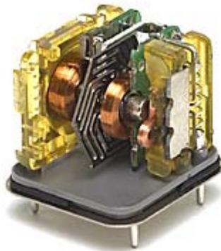
**Fig. 66 - Cut through of a micro gyro from Gyration [14]**
