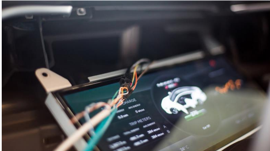
Figure 12: Connecting an Ethernet cord to the dashboard and gain access to the vehicle.
