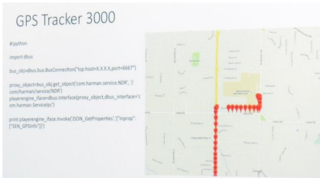
Figure 9: How GPS tracking was used to determine which Jeep Cherokee was their target vehicle.
