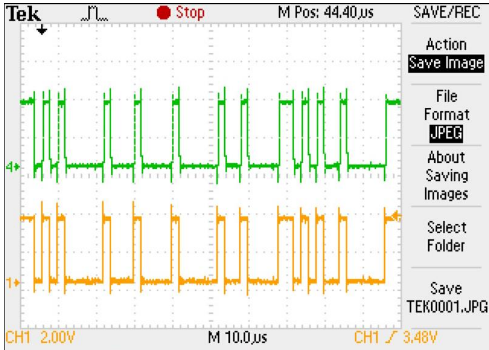
Figure 35: Oscilloscope reading from the Data Logger with the BeagleBone Black. The yellow signal is the CAN packet from the BeagleBone Black and the green signal is the CAN packet at the Rx pin of the Teensy.
