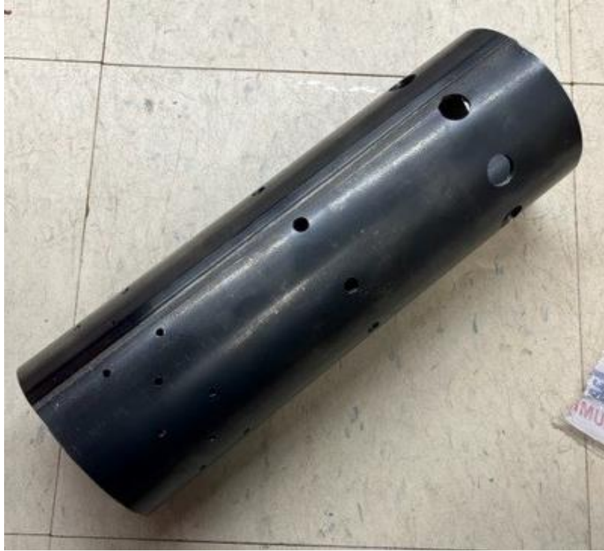
Figure 14: Flame tube with Holes Pressed
