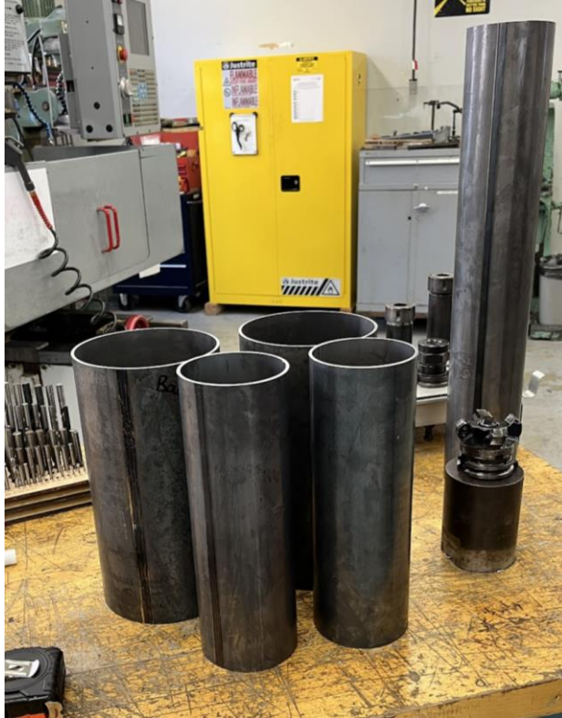
Figure 13: Flame Tube and Cover Tube Cut to Size Using the Horizontal Band Saw
