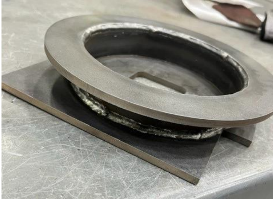
Figure 16: Adaptor Piece Welded to Two Plates
