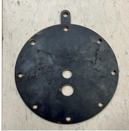
Figure 12: Plate Cover Cut by the Water Jet
