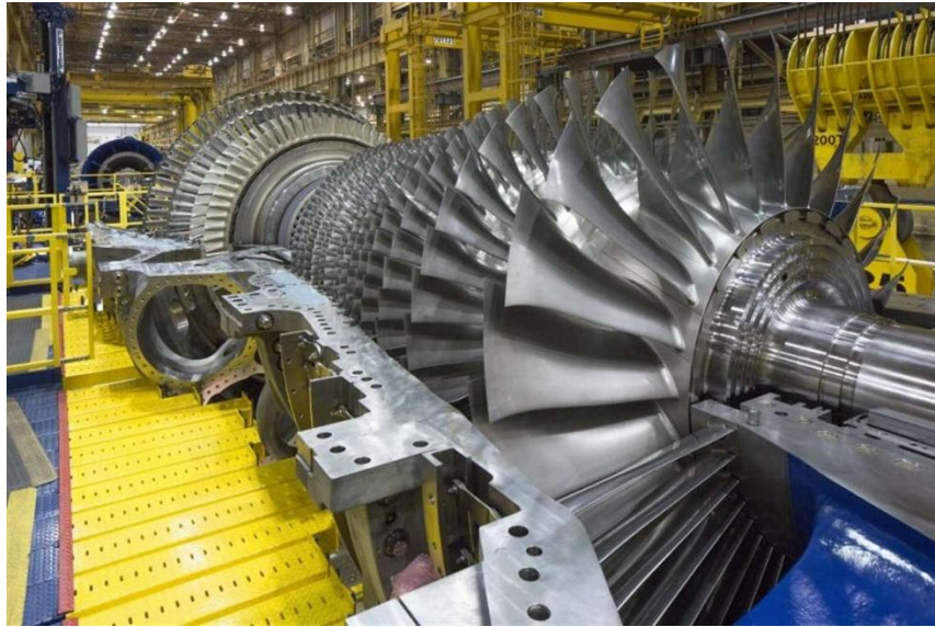
Figure 4: General Electric Gas Turbine Generator
