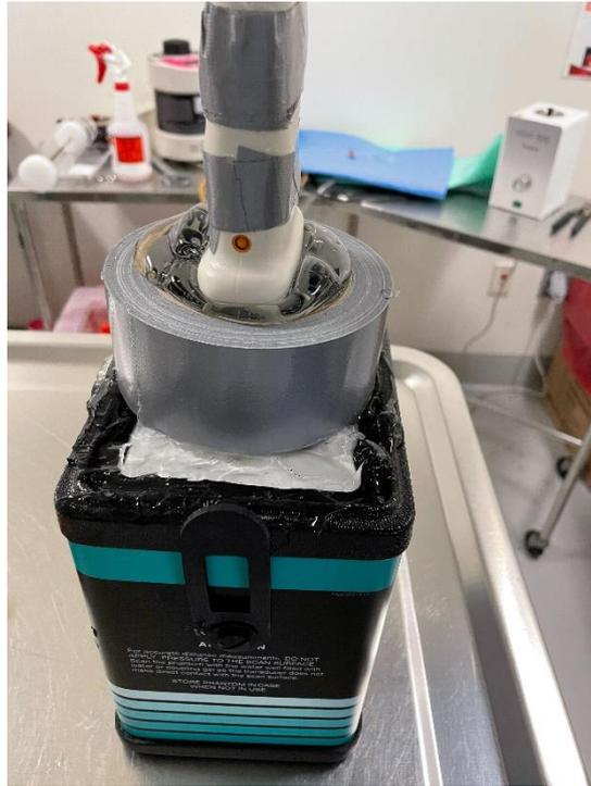
Figure 57: Base line data collection using just the US transducer and the gel medium. The roll of tape was used to prevent US gel from spilling in the test area.
