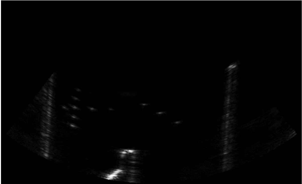
*Figure 45: Cross section image collected from phantom test with only the probe. The dots are the known markers in the phantom.*
