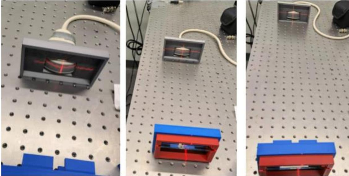
*Figure 41: Laser Alignment testing showing the laser crosshair signal with successful alignment at short and intermediate distances, and slightly out of alignment at the longest distance.*
