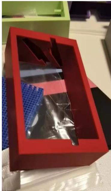
*Figure 25: Printed prototype with newly implemented recessed slot solution to mirror support and securement.*
