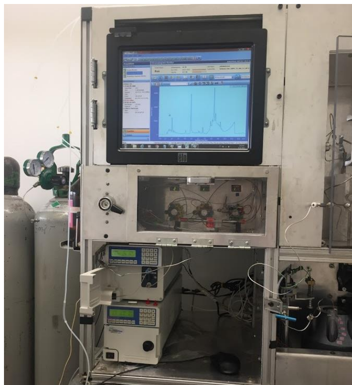
C.2: Laboratory Photograph of HPLC Machine made for HMF and FF Detection
