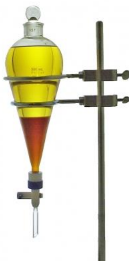
Figure 3-8: Biodiesel Settling in Separatory Funnel
