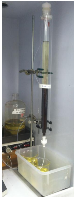
Figure 3-9: Resin Column refining dealcoholized biodiesel
