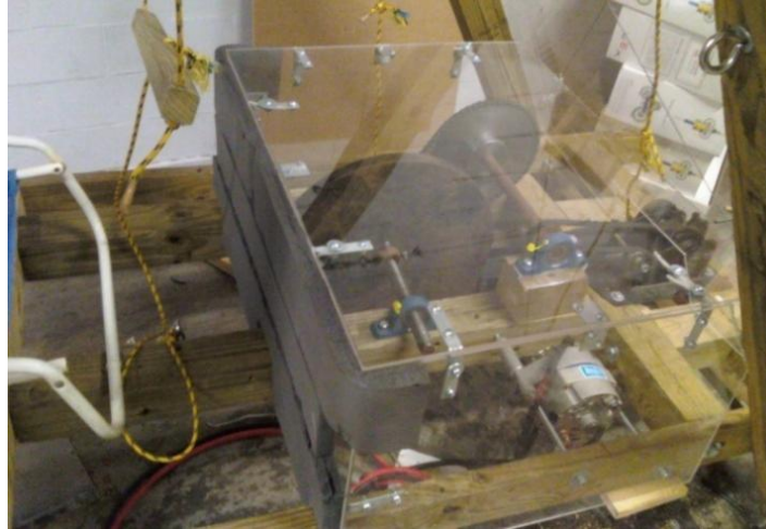
Figure 39 - Modified Acrylic Enclosure covering the gearing
