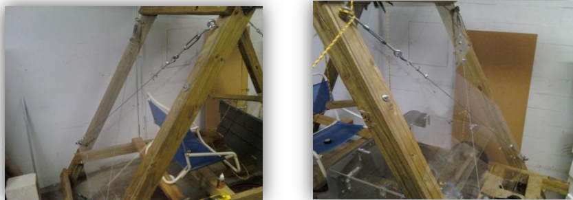
Figure 40 - Acrylic Panel on Front and Rear of A-frame
