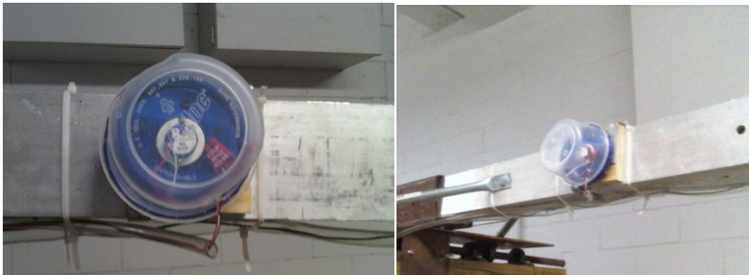
Figure 21 - Final Setup of Inclinometer on the Rocking Arm
