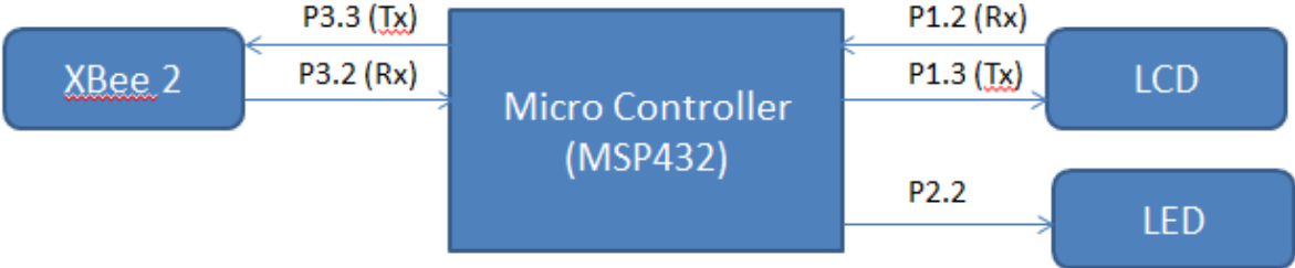
Figure 3.4: Base Station Block Diagram
