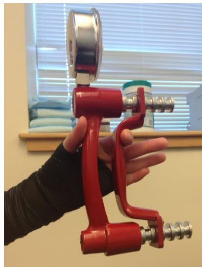
Figure 46: Hand dynamometer pinch testing with splint
