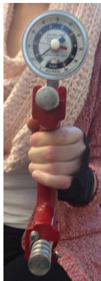
Figure 43: Hand dynamometer team testing front view
