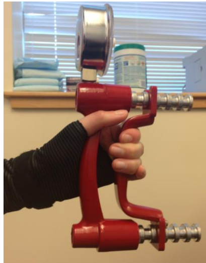
Figure 45: Hand dynamometer grip testing with splint
