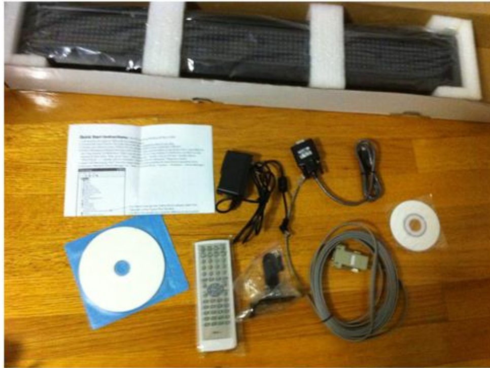
Figure 9: The additional contents and the scrolling LED sign. The contents include one page of instructions, a mini-CD with drivers, a regular CD with software, the power adapter, the USB-to-RS-232 adapter, the RJ25 connector, the remote, and the fixtures that can be used to mount the LED sign.
