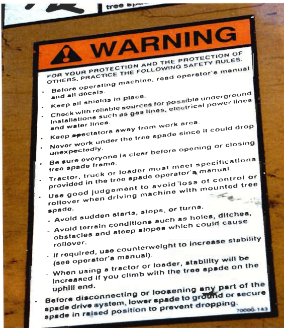
Figure 6-4. Safety Warnings On The Tree Spade.
