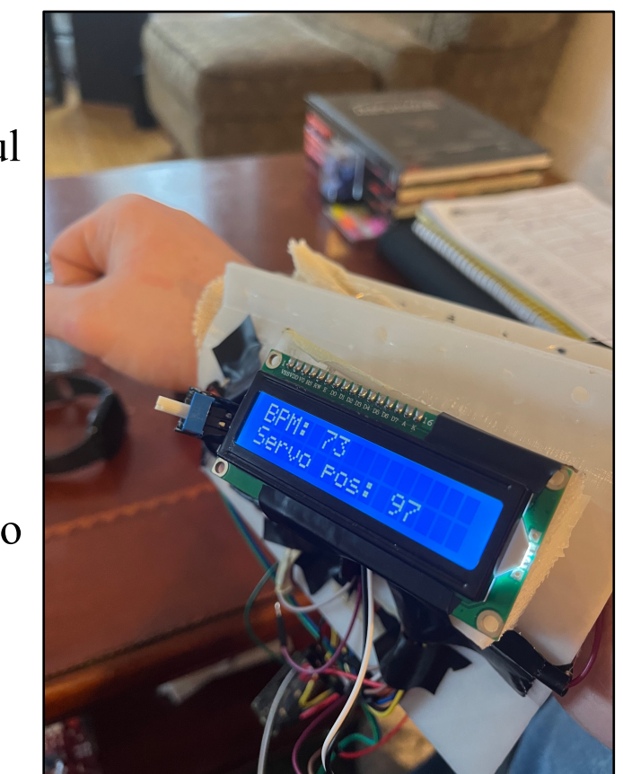
Figure 6: Arm Cast Placed on Achilles' arm performing a tightening calibration to return to baseline tightness
