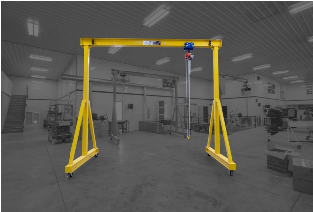
Figure 9: Overhead Gantry Crane
