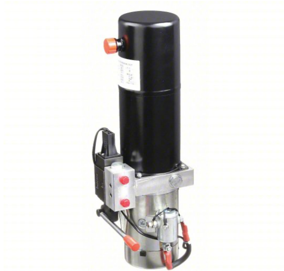
Figure 26: MAXIM Hydraulic Power Unit: 1.3 gpm, 2,500 psi Max. Pressure, 0.75-gal Reservoir Capacity, 12V DC
