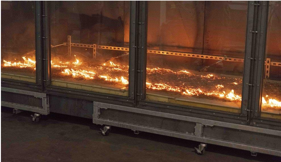
Figure 3: Fire-Testing in the FPE Wind Tunnel
