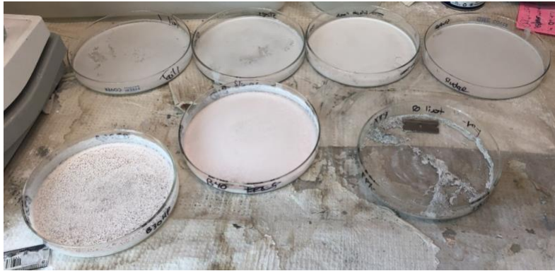
Figure A- 5: Petri dishes with micronized samples after drying overnight. One sample has been scraped with a razorblade and partially removed from its petri dish.
