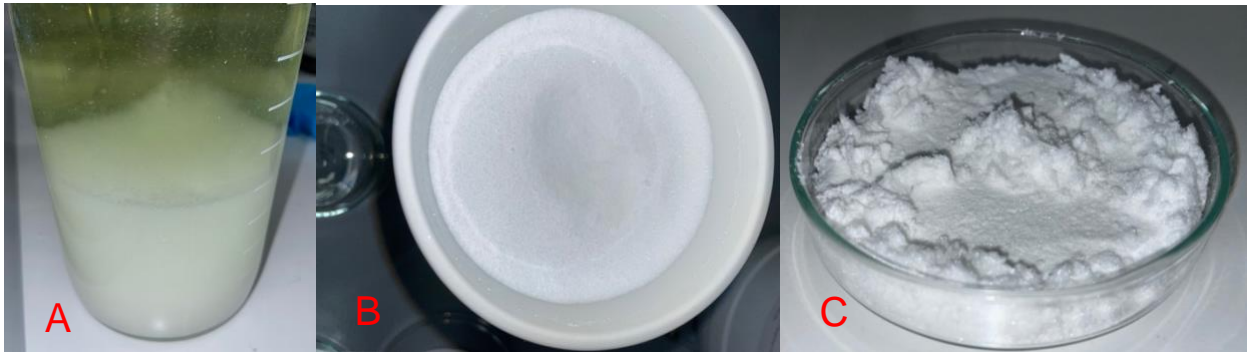
Figure A- 20: Ammonium oxalate precipitated during carbonation of oxalic acid extraction solutions, (a) in solution, (b) in filter, and (c) after overnight drying under fume hood
