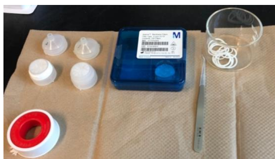
Figure A- 9: Materials for flow-through reaction chamber. Top left to right: two chambers, with lids sitting above bottoms; box of 0.2 \mu\text{m} filters; tweezers; beaker containing rubber gaskets. Bottom left: polytetrafluoroethylene (PTFE) tape to seal chamber threading. (The chamber bottom on the left is shown with tape wrapped around threading.)
