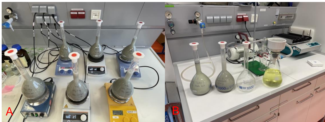
Figure A- 15: Experimental setup for (a) alkalinity extraction via acid dissolution and (b) vacuum filtration
