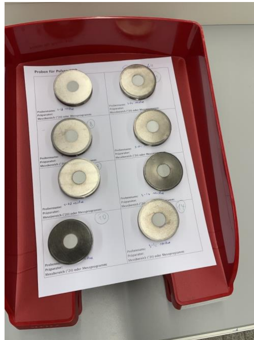
Figure A- 18: Back-loaded mounts for quantitative XRD measurements
