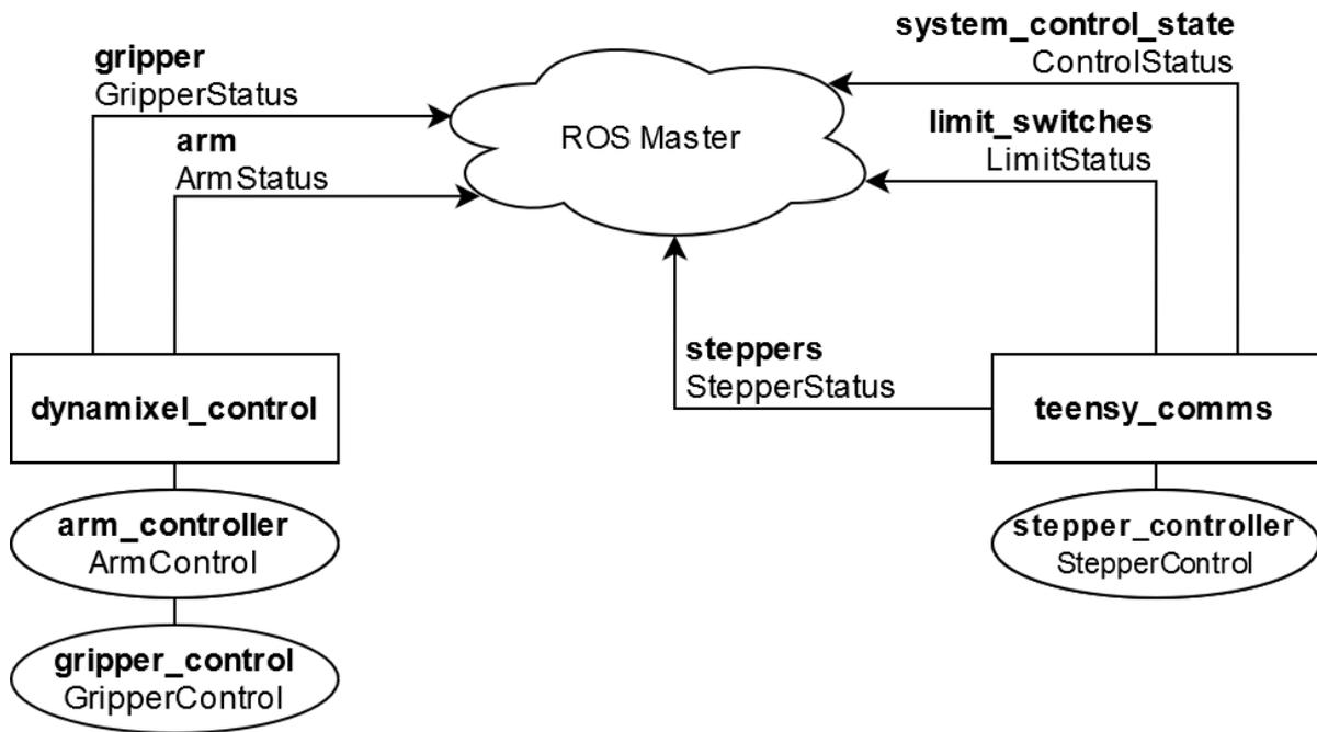
**Figure 4.7:** ROS Nodes shown as rectangles. Messages are illustrated using arrows indicating publishing, labeled with the bolded name and message type. Services are illustrated using ellipses, labeled with the bolded name and service type.
