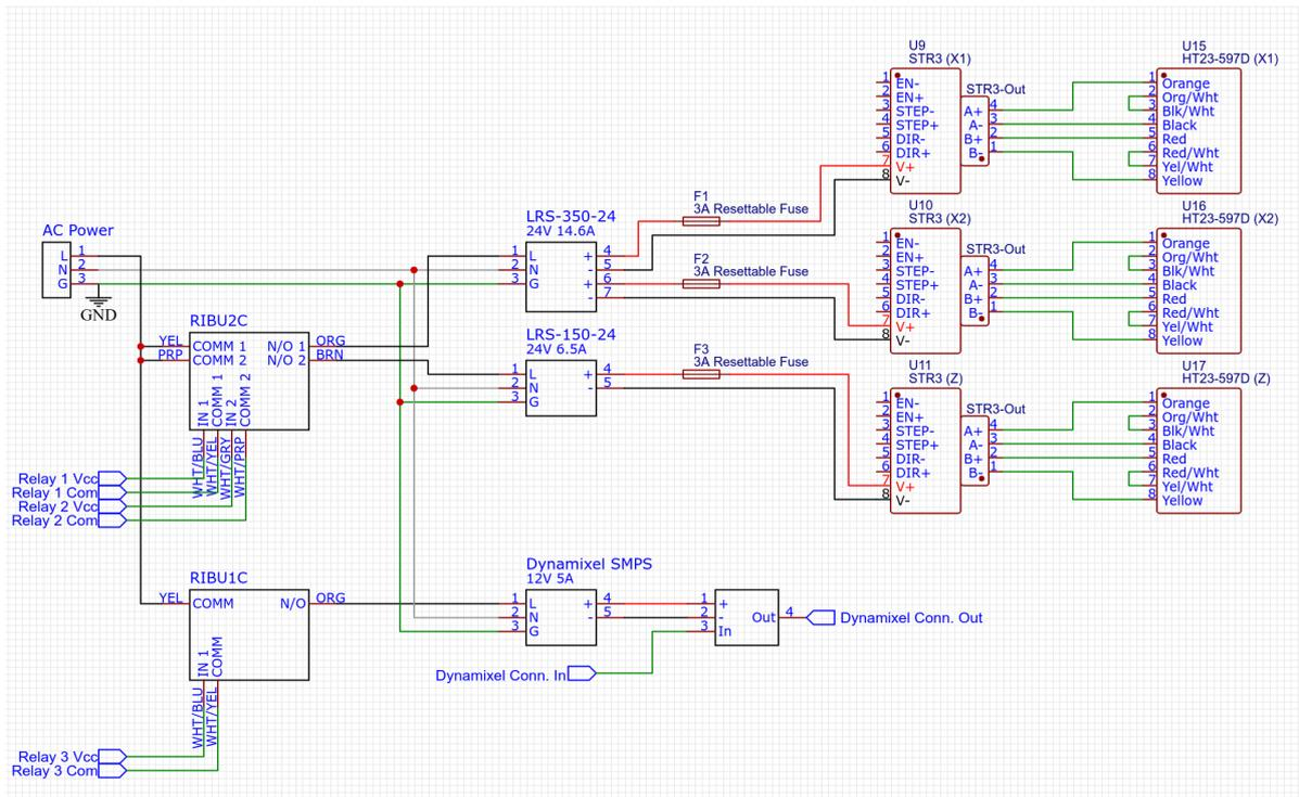
**Figure 3.5:** Motor Power Distribution. Ground is common to all devices.
