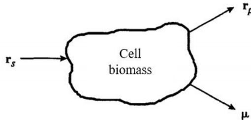
**Figure 1:** Diagram of the black-box model, where  $r_s$  is the rate of substrate uptake,  $r_p$  is the rate of product formation and  $\mu$  is the accumulation of biomass [18].
