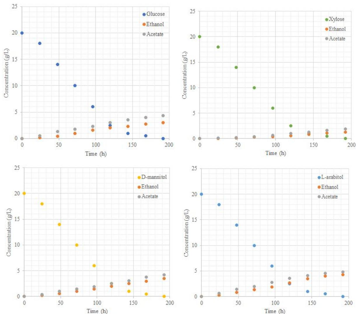
**Figure 6:** Plots showing sample raw data from enzymatic kits measuring the concentration of the carbon sources (glucose, xylose, L-arabitol, and D-mannitol) and by-products (ethanol and acetate) in the fermentation of *K. xylinus* in HS media. All plots contain sample data for demonstration purposes only.
