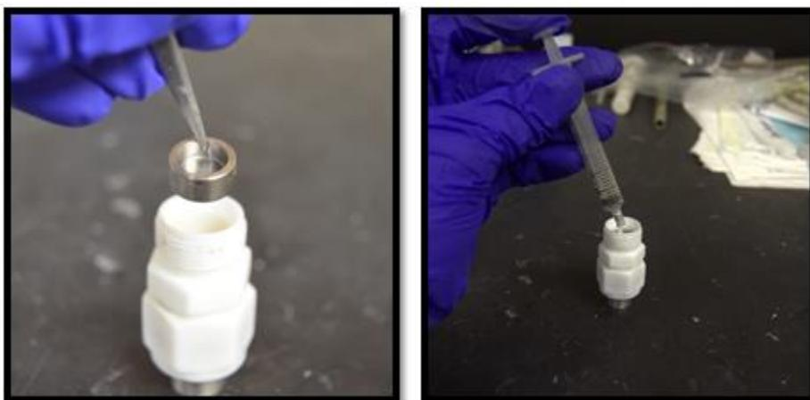
Figure 46: Addition of stainless steel crucible to top of compression spring (left). Addition of liquid gallium to the crucible using a syringe (right).
