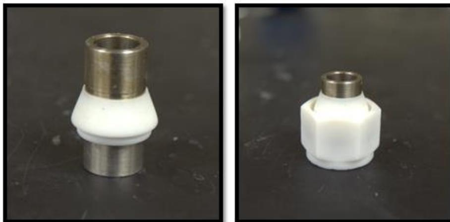
Figure 44: Ferrule orientation on anode current collector (left) in Swagelok PTFE fitting (right).
