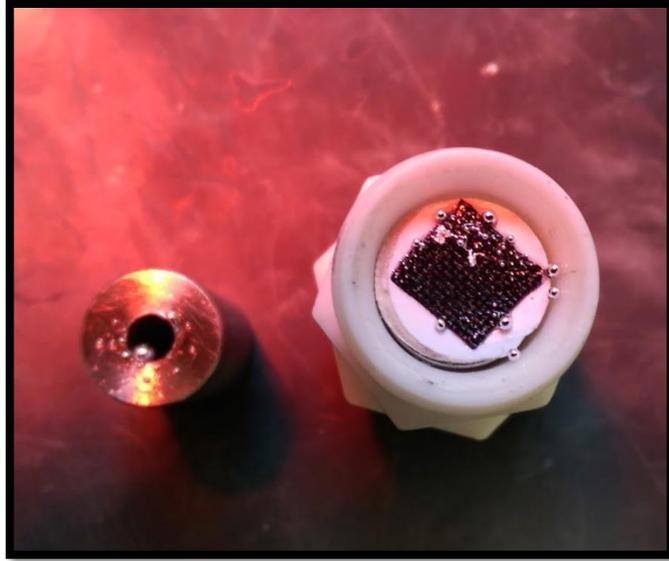
*Figure 30: Image of a short circuited cell attributed to gallium leakage*
