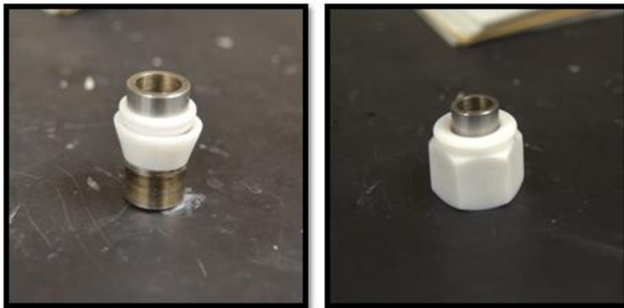
*Figure 49: Ferrule orientation on air cathode current collector (left) with Swagelok fitting added (right).*
