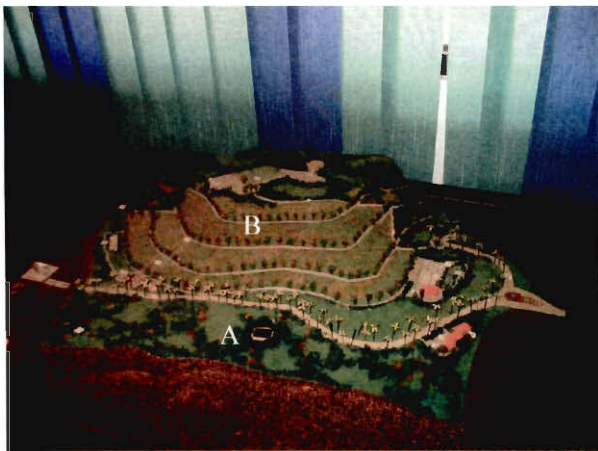
Figure 9: Model of Río Azul after being closed and capped. Notice the small black rectangle (A). That is the lagoon that is meant to hold the leachates produced by the entire landfill above (B).
