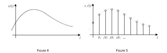
The <u>Nyquist frequency</u> is half the sampling frequency of a discrete signal processing system, sometimes referred to as the folding frequency. The Nyquist frequency is not the same as the Nyquist rate. It is important to understand that this frequency is a property of a discrete-time system, not of a signal. The Nyquist rate, however, is a property of a continuous-time signal and not of the system responsible for recording (sampling) it. (Source: 1)
