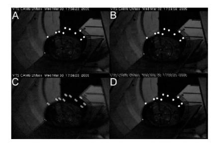
Figure 15 - A. Phantom before camera motion. PTZ parameters are saved. B. Phantom after camera was moved, rebooted and reoriented using saved PTZ parameters. C=A+B. Notice imperfect overlay. D=A+(B corrected). Overlay is almost perfect. [20]
