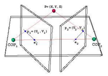
Figure 26 – Stereo Computation with Triangulation [39]
