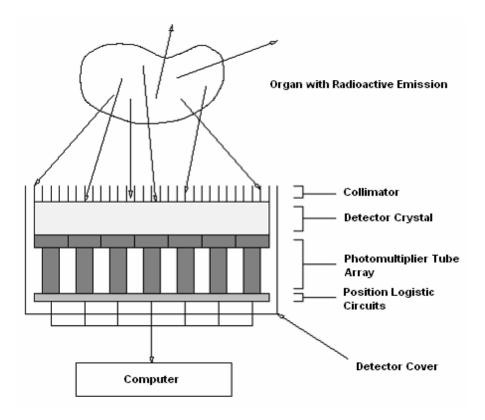
Figure 1 - SPECT Imaging Using a Gamma Camera [6]
