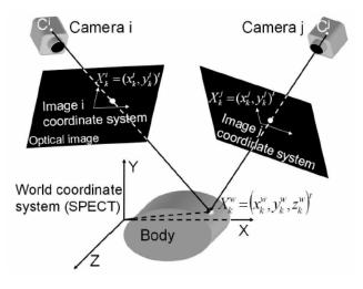
Figure 14 – Coordinate Systems for VTS and SPECT. The lines  $(C^i, X^i)$  and  $(C^i, X^j)$ intersect at  $X^w$  [20].
