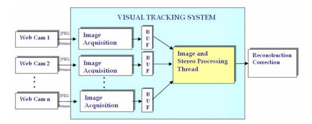
Figure 9 – Software Architecture Design on the VTS System [4].
