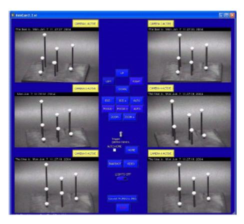
Figure 8 – GUI of the VTS system looking at the calibration phantom in 6 views [15].
