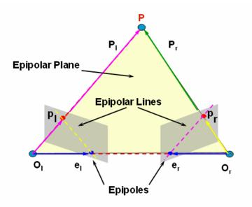
Figure 17 - Epipolar Geometry of a Stereo System [19].
