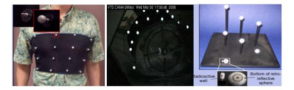
Figure 5 – Left - One version of Stretchy Garment design with Reflective Spheres, Center – Asymmetrical version of the Garment, Right - Calibration Phantom [15].
