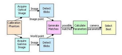
Figure 12 – Calibration Processing Flow [18].
