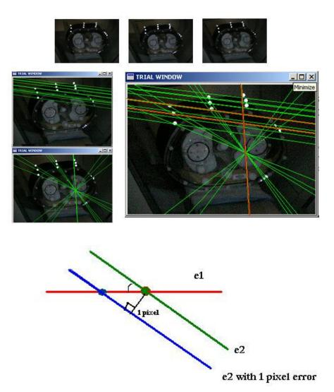
Figure 19 – Case of epipolar line overlaps (marked in red). Top – three views at a particular instant, Left – Epipolar projections 1 to 3 & 2 to 3, Right – Intersection of Epipolar lines, the overlapping lines make it hard to find the right match. Bottom –
