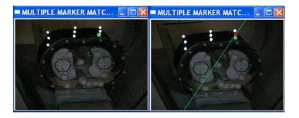
Figure 23 – Epipolar line projection showing possible wrong match
