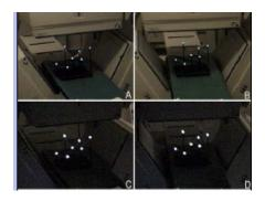
Figure 6 – Calibration Phantom on the SPECT table with and without lights on [15].
