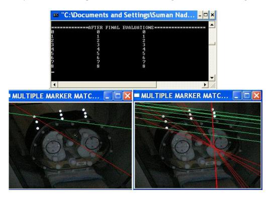
Figure 25 – Top - Final Evaluation Results, Left - Intersecting epipolar lines for feature 0, Right - Visualization of all markers of 1 and 2 projected onto 3
