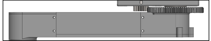
Figure 27: SolidWorks model of the first link separated into three pieces
