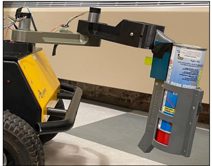
Figure 21: Marking solution from previous MQP team
