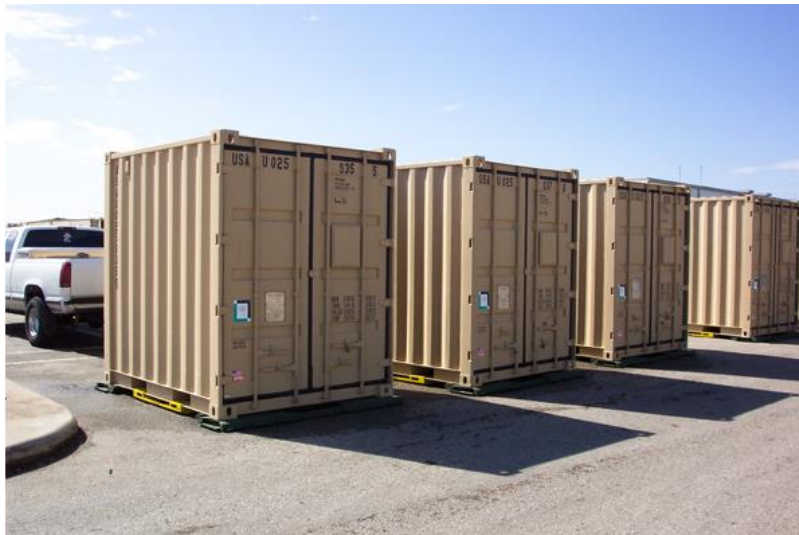
Figure 4: Various 8'x'6.5'x8' TRICON containers (CMCI, 2011)
