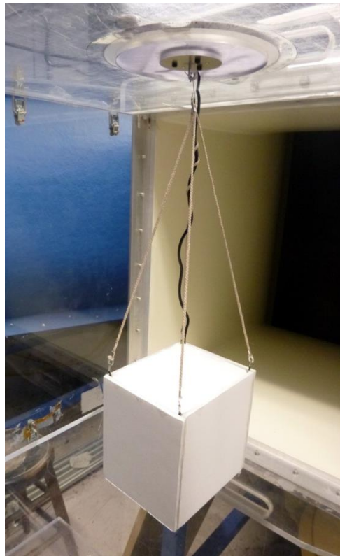
Figure 29: Poster-board TRICON (note power cord - this was removed for subsequent tests)
