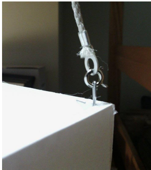
Figure 31: Detachable Sling Legs on the Second TRICON Prototype
