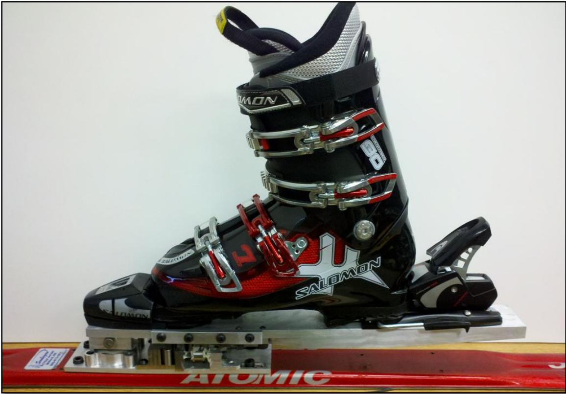
Figure 33: Under-binding plate assembled with binding mounted
