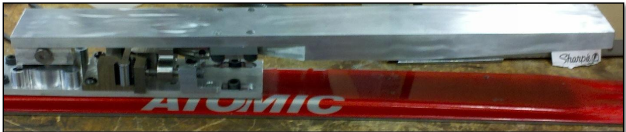
Figure 32: Under-binding plate assembled on ski
