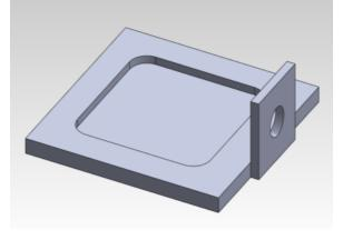
Figure 40: SolidWorks Representation of Layered Acrylic Base
