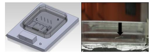
Figure 1. (left) SolidWorks<sup>™</sup> drawing of preliminary design for mechanical stimulation (right) Assembled device with tissue construct (black arrow) mounted on pins
