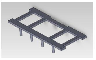
Figure 42: Slider with Mounting Pins and Notch for Magnet
