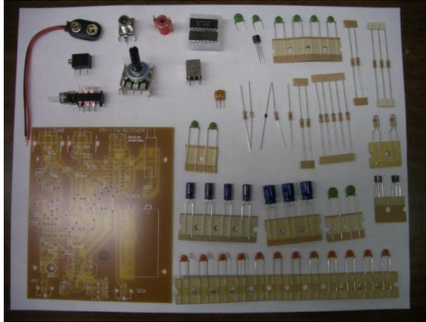
**Figure 65: Unassembled Radio Receiver**
