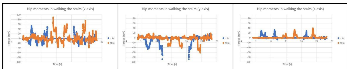
Figure 7: Hip moments in stair walking motion around the x-, y-, and z-axis, respectively.
