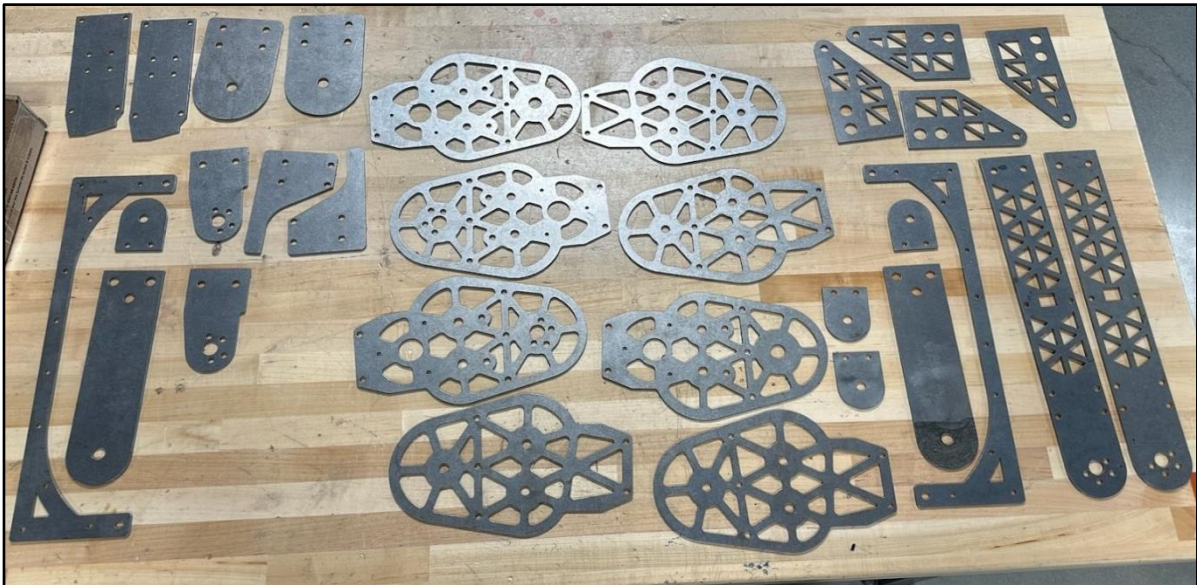
Figure 34: Hydro cut plates
