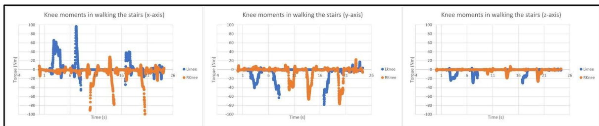
Figure 6: Knee moments in stair walking motion around the x-, y-, and z-axis, respectively.
