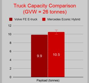
Figure 12: Comparison of the Volvo Etruck and Mercedes Hybrid Capacity Capabilities<sup>11,12</sup>
